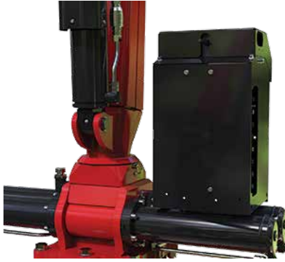
Electro-proportional control Danfoss with console and 2 joysticks
