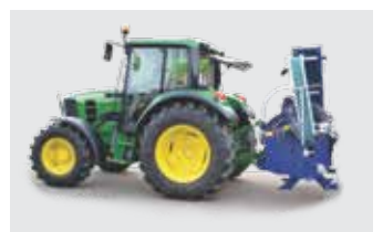
Transport position: In-feed and Discharge Conveyor, as well as the Log Loader can be set against the machine and attached. The machine is mounted to the tractor using three-point system.
