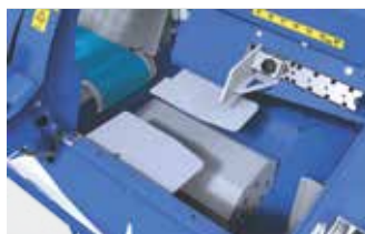
Two Swinging Laps remain in the horizontal position during cutting. Once the log is cut, the laps open and the log falls into the splitting chute.
