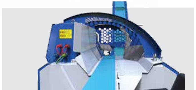
Before the Hydraulic Log Holder there is a Guide Lean that guides the log and prevents it from hitting the log holder. The Hydraulic Log Holder is used to fix the log and prevent it from spinning and turning.
