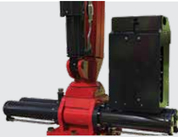
8-section electroproportional hydraulic valve allows precise control with control console.
