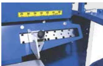
The Hydraulic Length Limiter with offset function can be set from 25–50 cm.
