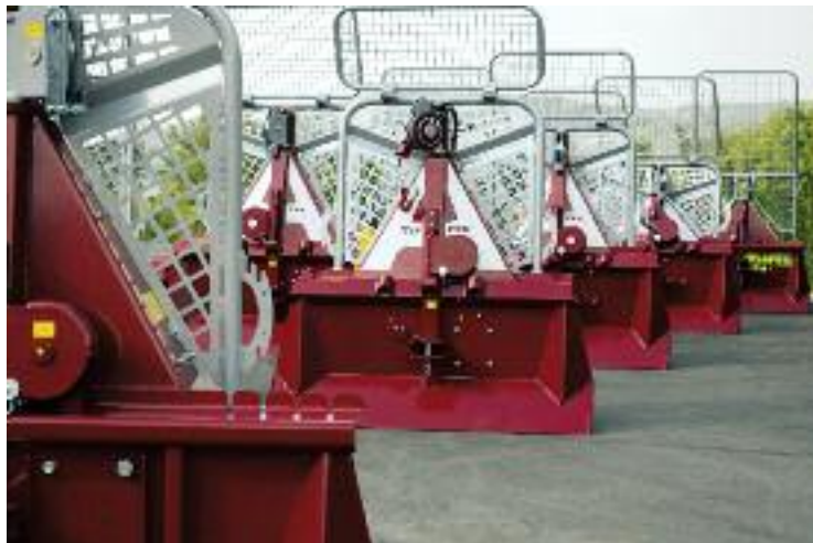
Logging winches ready for delivery
